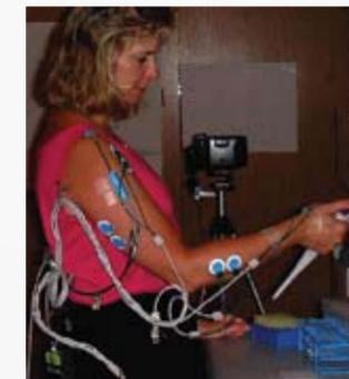
EMG (electromyogram) testing was used by VistaLab to measure the activity and stresses of pipetting on five muscle groups when using traditionally shaped pipettes, and then compared to the Ovation design. This testing was done during the development process for the Ovation Pipette in 2001.
