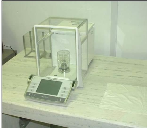
Figure 3: Setup used to weigh 10mg samples with an evaporation trap.
