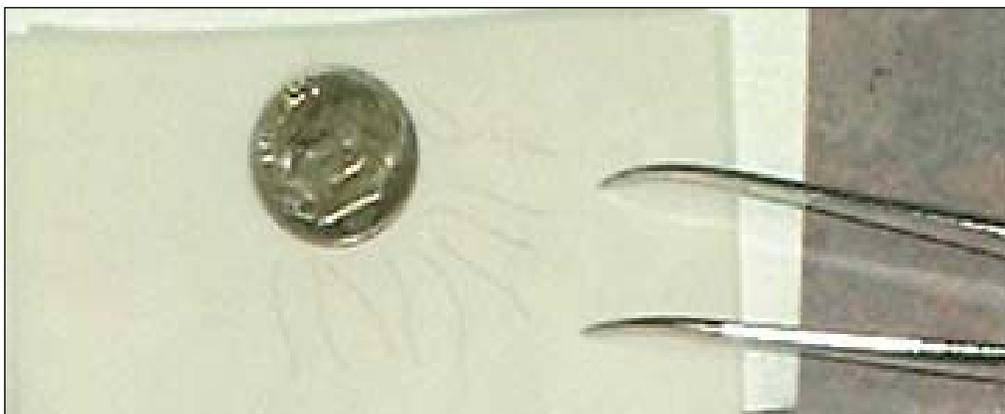
Figure 12: Wire artifacts used for straight addition weighing method.
