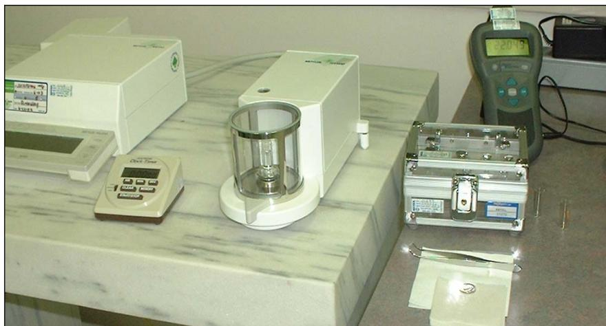
**Figure 11: Setup used to weigh 200 $\mu$ g samples in the presence of humidity controls.**
