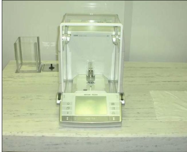
Figure 9: Setup used to weigh 10mg samples in the presence of humidity controls.
