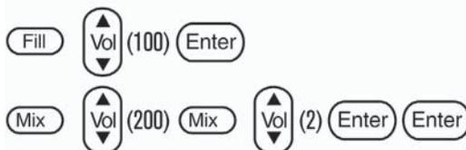
After pressing the final Enter key, you are now ready to pipet. Each time you squeeze the trigger, the next step of the program will initiate. You can also save up to six of these programs (up to 40 steps each) in memory, so they are quickly available the next time you need to use them.
