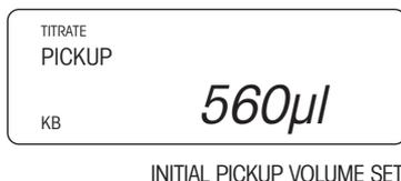
2. To set an initial dispense volume, press number keys then press **E** . (To set an initial dispense volume without changing the initial pickup volume, press **E** first. Enter the volume with number keys. Then press **E** again.)
