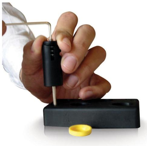
5. Turn the volume dial to the average volume determined by weighing.
